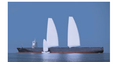
Wisamo, an inflatable, retractable and automated wing sail, will be tested on the Compagnie Maritime Nantaise's ro-ro container ship MN Pélican
